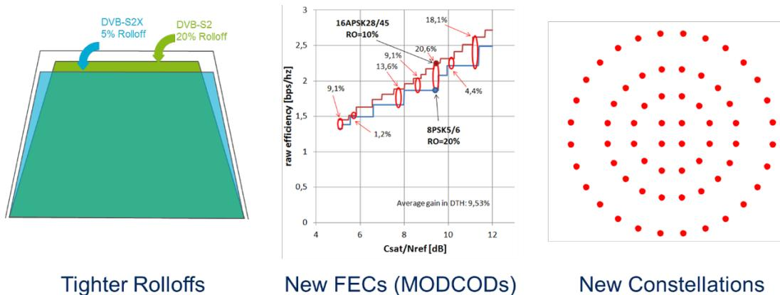
FIGURE 1 – NEW DVB-S2X TOOLS TO IMPROVE TRANSMISSION EFFICIENCY
