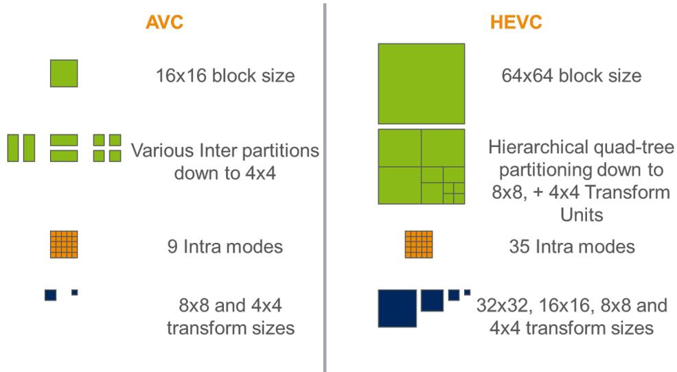
FIGURE 2- COMPARING MPEG-4 AVC AND HEVC TRANSFORM MODES
