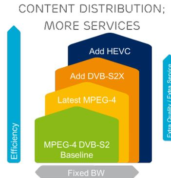
FIGURE 7 – HOW DVB-S2X AND HEVC CAN COMBINE TO ALLOW MORE REVENUE GENERATING SERVICES WITHIN AN EXISTING BANDWIDTH/OPEX IN THE DISTRIBUTION MARKET
