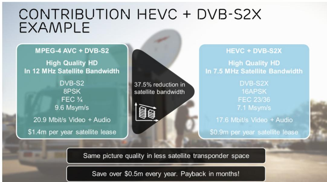
FIGURE 6 – SUMMARY OF LIKELY EFFICIENCY AND MONETARY GAINS IN CONVERTING FROM BEST-IN-CLASS DVB-S2/MPEG-4 AVC TO DVB-S2X AND HEVC IN A CONTRIBUTION SCENARIO
