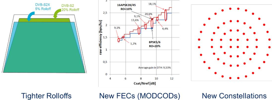
FIGURE 1 – NEW DVB-S2X TOOLS TO IMPROVE TRANSMISSION EFFICIENCY
