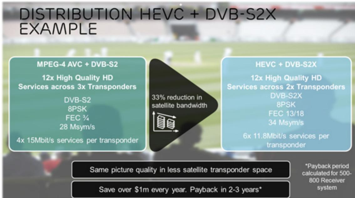
FIGURE 10 – SUMMARY OF LIKELY EFFICIENCY AND MONETARY GAINS IN CONVERTING FROM BEST-IN-CLASS DVB-S2/MPEG-4 AVC TO DVB-S2X AND HEVC IN A DISTRIBUTION SCENARIO
